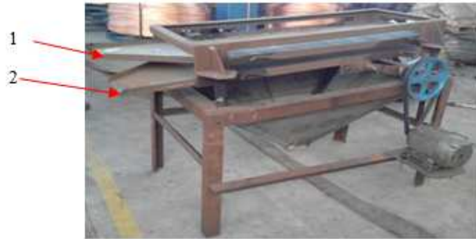
Fig. 6 Completed sieving mechanism design
