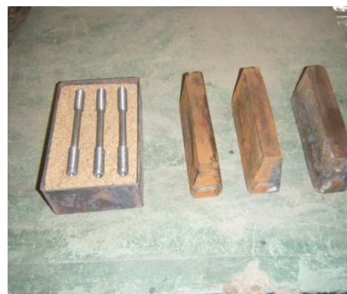
Fig. 12 Specimens for tensile test and Microstructure
