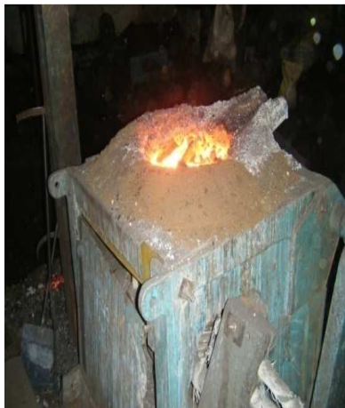
Fig.1 Electric induction furnace
