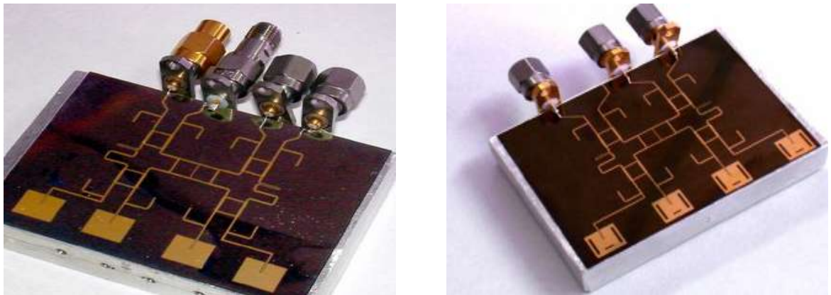
Fig.11 Single band assembly and dual band assembly on silicon [10]
