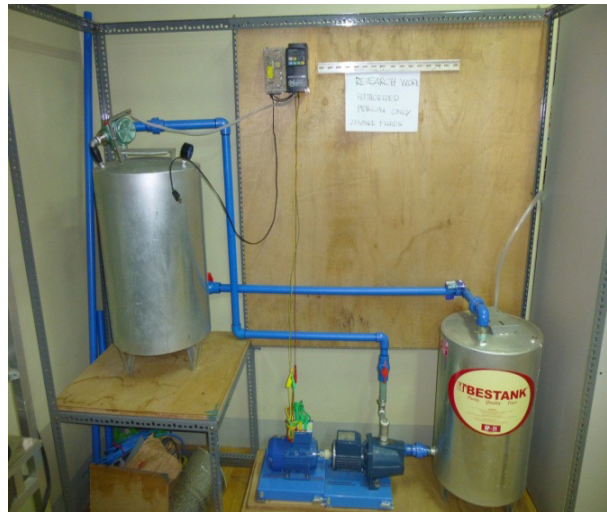
Fig. 2.5: Process Control Test Set-up
