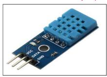
Humidity sensors work by detecting changes that alter electrical currents or temperature in the air. There are the basic types of humidity sensors: capacitive, resistive and thermal. All three types of sensors monitor minute changes in the atmosphere in order to calculate the humidity in the air.
