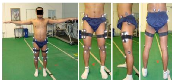
Figure 1: marker placement on participant; anterior view, anterior view close up, left lateral view and posterior view
