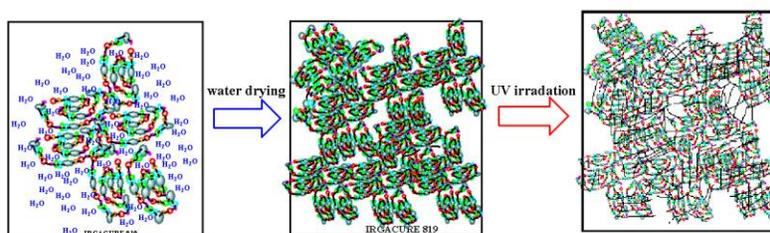
Figure 4: Film forming process of UV-PUA
