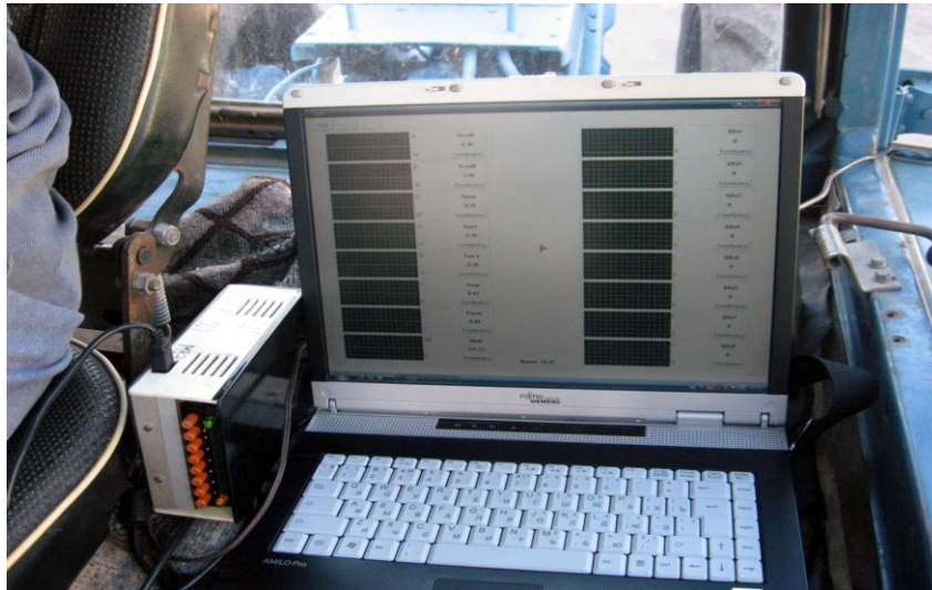
Fig. 5 – Arrangement of the recording complex in the tractor cab
