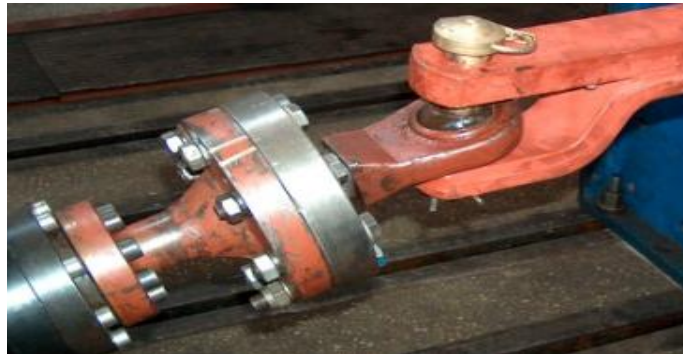
Fig. 4 - Mounting on the Hidropuls installation for the static test of the draught bar
