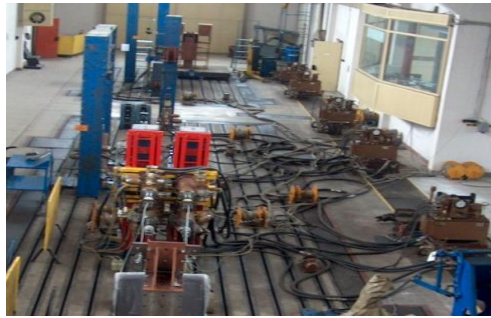
Fig. 3 – Testing installation in simulated and accelerated regime, Hidropuls type
