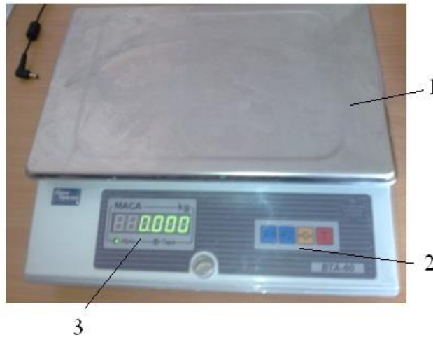
Fig. 2 - BTA-60 / 30-5-T Electronic laboratory technical balance 1 - weighing pan; 2 - panel calibration; 3 - display indicator
