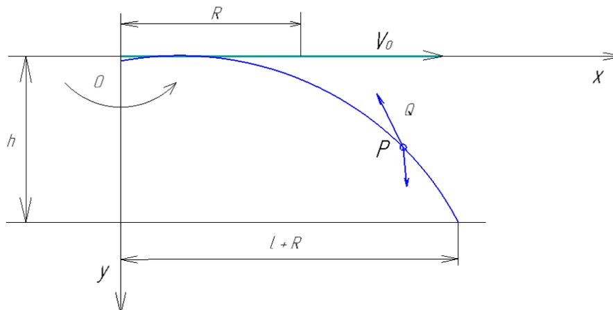
Fig. 6 - Diagram of granules flight analysis
