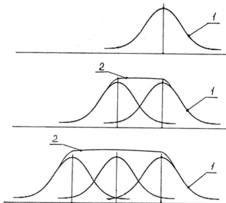
**Fig. 1 - Graphical interpretation of fertilizer granules distribution on the field surface in the presence of other (a) two (b) three and (c) vanishing points from a disk surface:**
