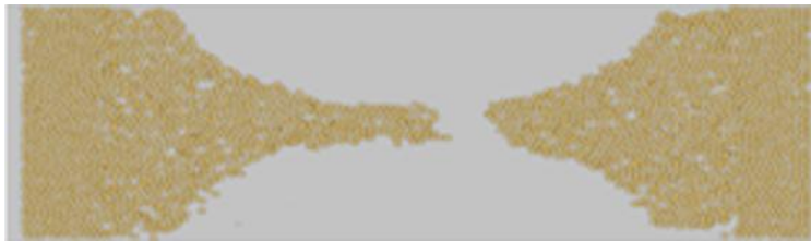
Fig. 10 - Simulated fracture surface of CSP specimen
