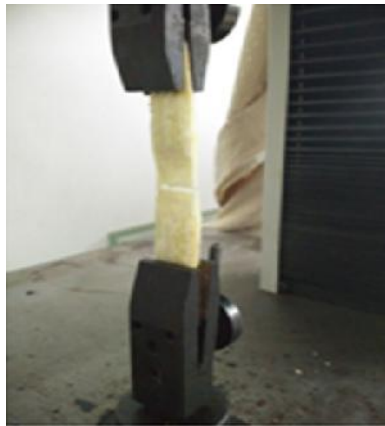
Fig.5 - The broken specimen
