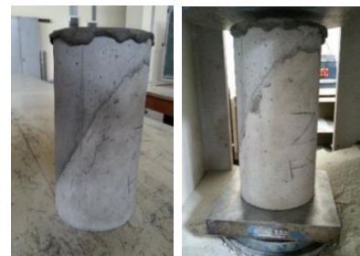
Figure 1: Specimens for slant shear test.
