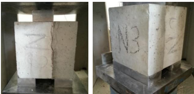
Figure 2: Specimens for bi-surface shear test.
