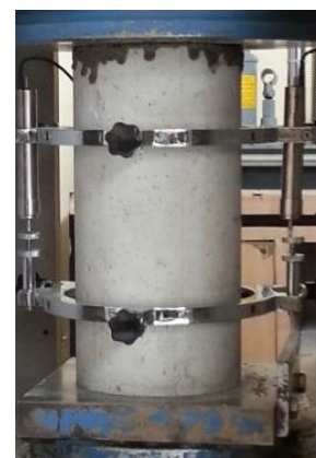
Figure 5: Composite specimens tested under uniaxial loading.
