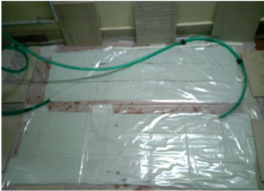
Fig. 2 – Vacuum Bagging Method.
