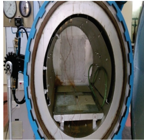
Fig 3. Laminates placed inside Autoclave.
