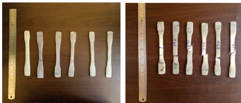
Fig. 4 – Tensile test Specimen before and after test.
