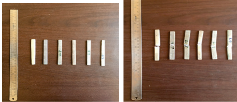
Fig. 5 – Flexural Test Specimen before and after Test.
