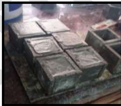
Fig 4.3. 70.7mm x 70.7mm x 70.7mm cubes
