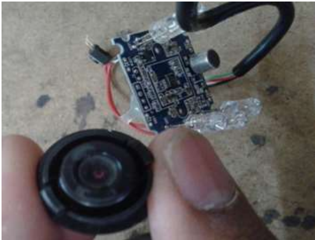
Figure.3 Lens assembly inside camera
