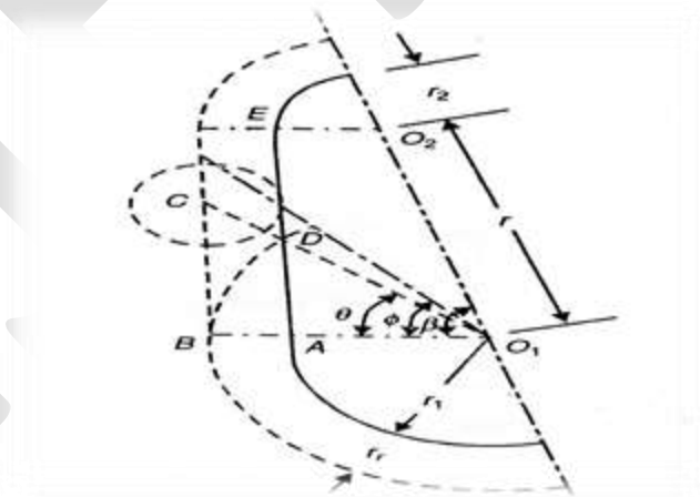
Fig.1. Tangent cam with roller follower in contact with straight flank[3]
