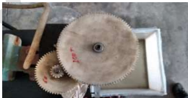
Figure6. Gear arrangement for speed reduction.
