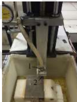
1. Electrolyte inlet, 2. Electrolyte outlet
