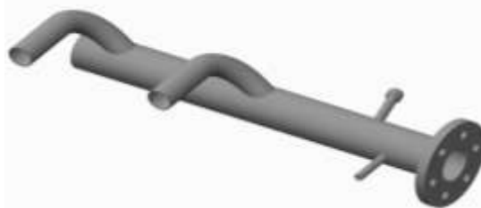
Fig. 1: 3D Parametric Model of Inlet Header
