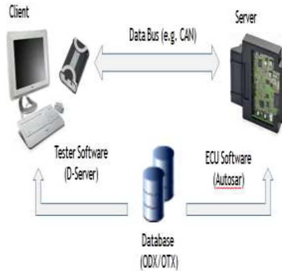
FIGURE 4: Basic structure of a diagnostic system[2]
