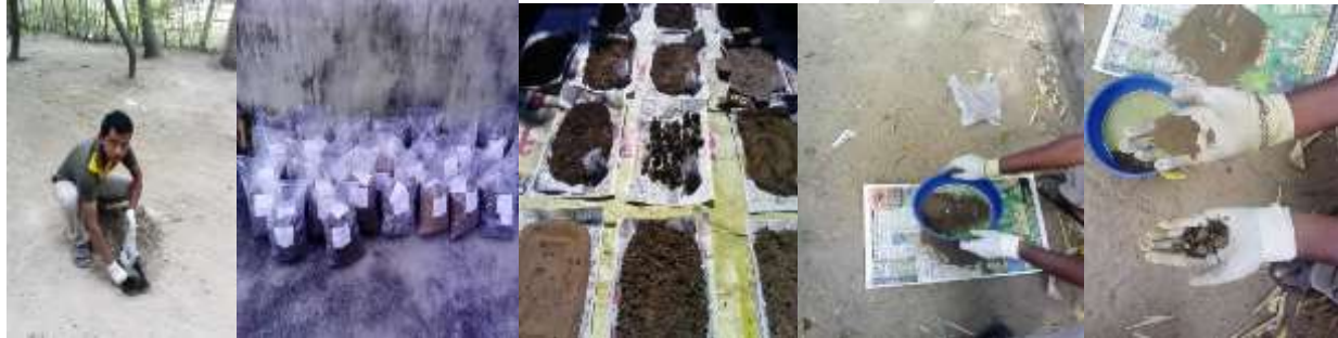
Fig 8: Soil sample collection, labelling, Drying, Sieving and removing other particles from sand
