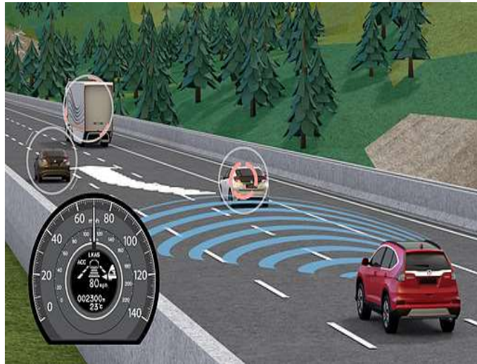
Figure 1. Adaptive Cruise Control using Radar based systems
