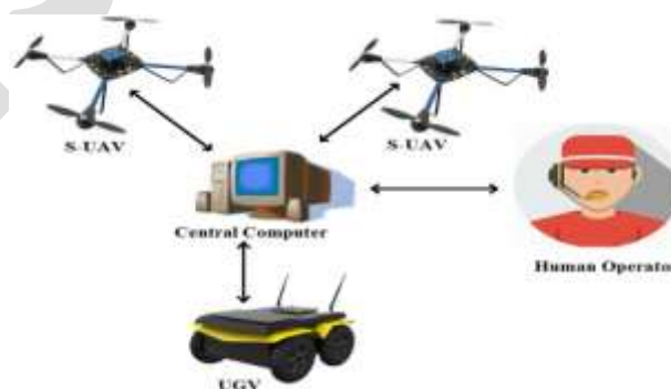
Figure 2: General structure of the proposed system
