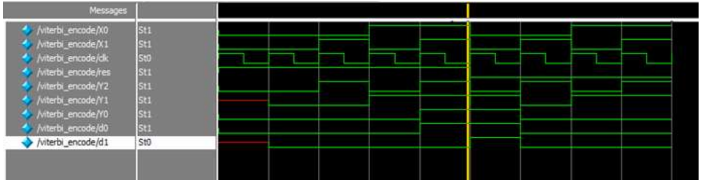
Figure4. Simulation of convolutional encoder
