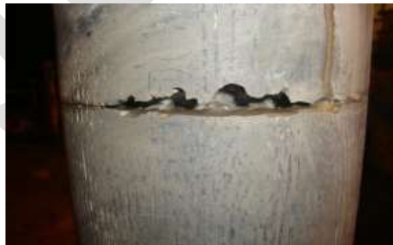
Fig. 2. Drill collars failure in Okono-9 offshore Niger Delta due to PDC Bit Vibration. Courtesy: NPDC, 2013.
