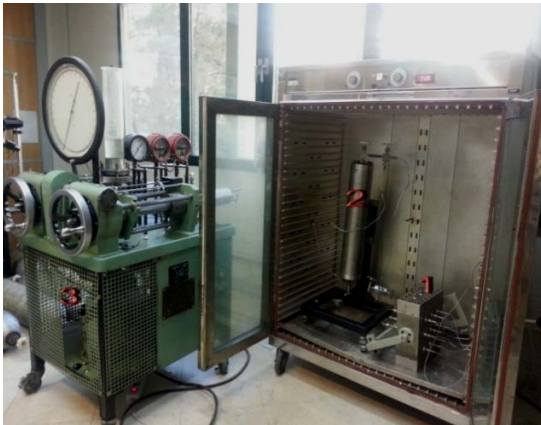
Fig. 3. Oil saturating set up; a) put the packed model inside the oven, b) fill the accumulator (600 ml) with heavy oil, c) connect the accumulator to injection pump and packed model, d) pump 2PV of heavy oil to the model to make sure it saturated with heavy oil completely.
