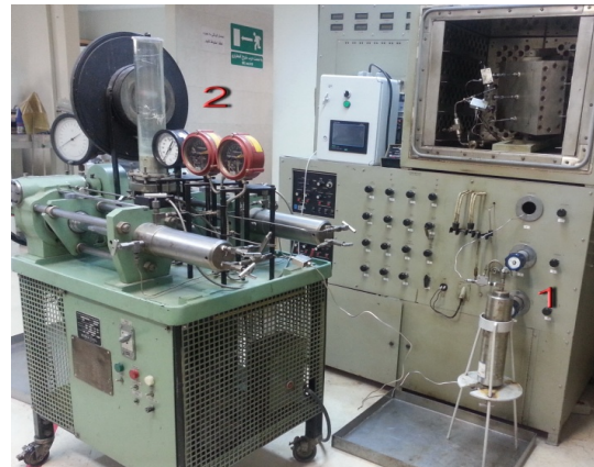
Fig. 4. Flooding the packed model with nanoparticles; a) fill the accumulator 600 ml with homogeneous ZnO nanoparticles solution, b) connect the accumulator to injection pump and packed model, c) pump 2PV of nanoparticle and flood the model.
