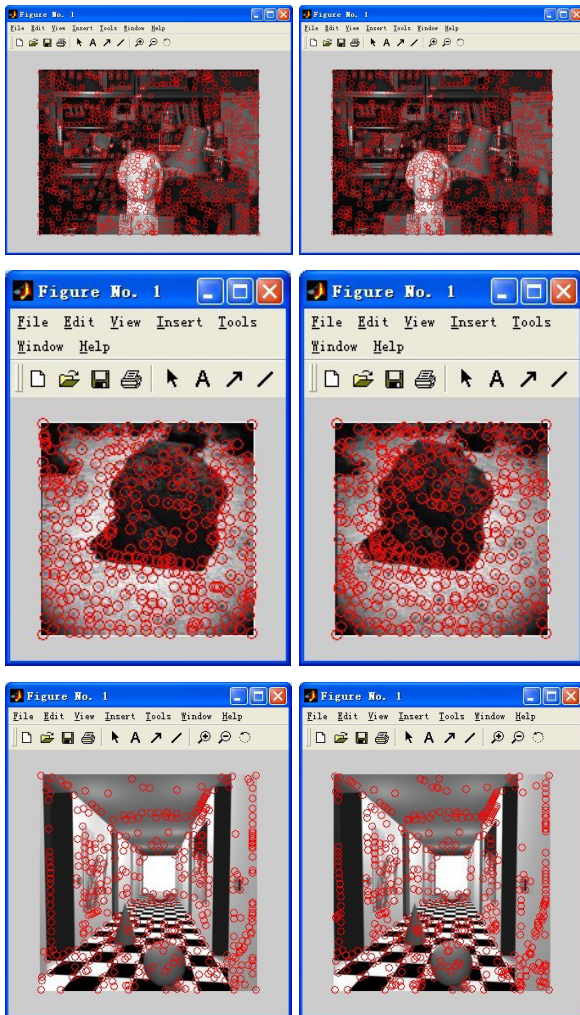
Figure 1 Detection result of harris operator
