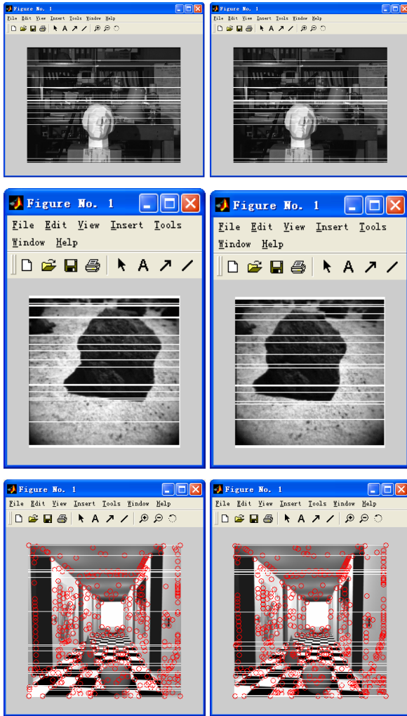
Figure 3 Restored polar line of feature points that false matching points are eliminated
