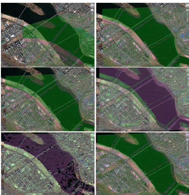
Fig. 11. Overlapped images in Aerial sets(Aerial 1)(Left – Up: FFT, Middle : Window, Bottom : Block Right – Up : Edge-FFT, Middle : Feature-point, Bottom : proposed).
