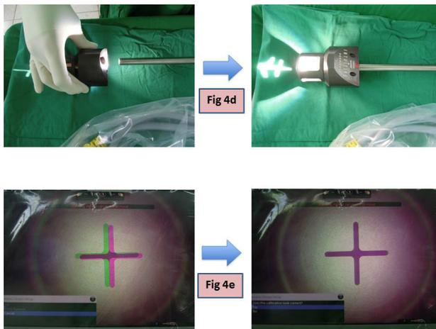
**Fig 4d-4e.** Endoscope alignment target for 3D calibration
