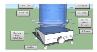
Figure 3. Gasifier Lower Assembly
