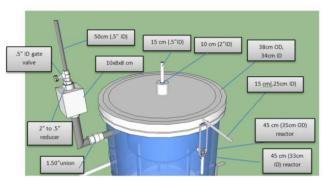
Figure 2. Gasifier Upper Assembly
