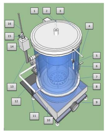
Figure 1. Isometric view of the Gasifier and its Parts
