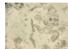
r. Broken fibres of Bambusa arundinacea
