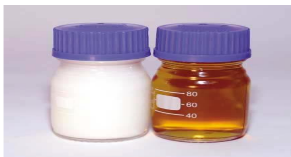
Fig 1: Difference between Emulsion and Microemulsion
