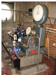
Figure 4 Engine brake SCHENK U116/2
