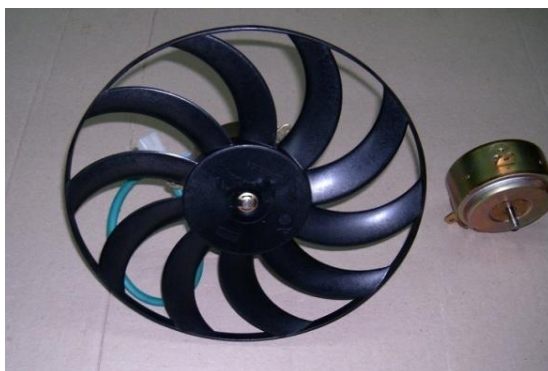
Figure 4 Final version of the new engine cooling fan motor [1]
