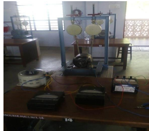
Figure 4 circuit arrangement for load test on single phase induction motor
