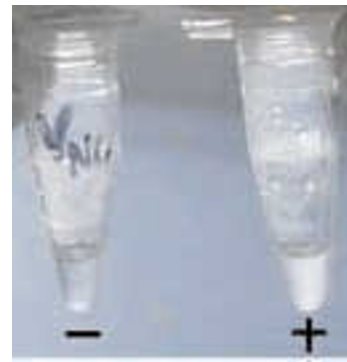
Figure 1. Differentiation of the LAMP reaction by visually observing the mixture for increase in turbidity. Left, without template (negative); right, with template DNA (positive). LAMP positive reaction produced an increase in turbidity of the mixture while the negative sample remained clear.
