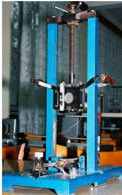
Foto 2. The stand for determining the behavior at impact
