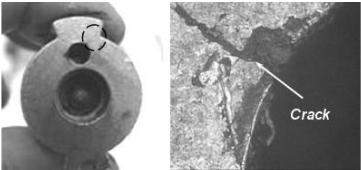
Fig. 11. Cracked torsional shaft of HKS.
