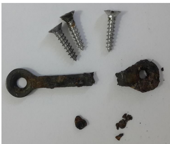
Fig. 2: Broken and corroded plate with screw after removal
