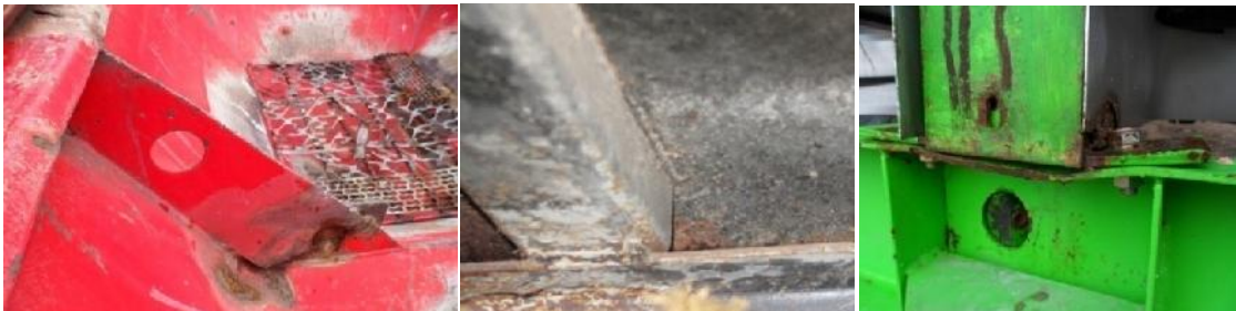
Fig. 1 – Corrosion-fatigue damages of fertilizer spreaders metal structures after two seasons of operation
