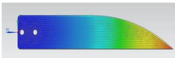
**Fig. 2 - Finite element analysis of the cutting edge**
