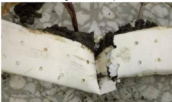
**Fig. 9 - Potted seedling after bending failure**
