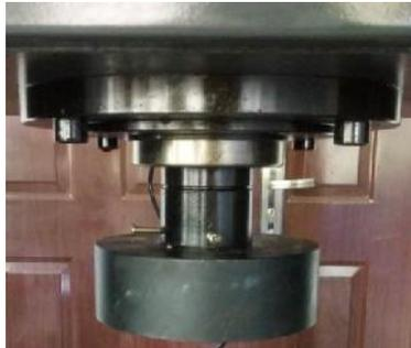
Fig. 5 - Bending cutter device
