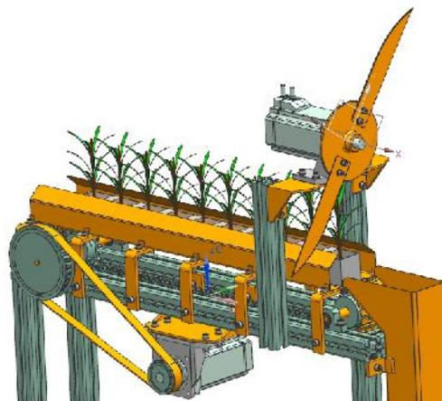
Fig. 1 - Three-dimensional assembly map of the seedling separator
