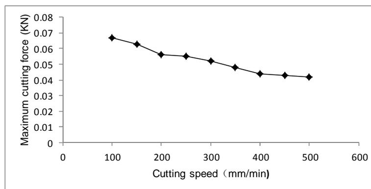
Fig. 12 - Variation of maximum cutting force with cutting speed
