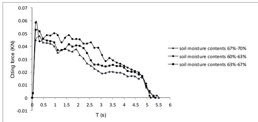
Fig. 11 - Variation of cutting force with time under different soil moisture contents
