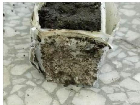
**Fig. 10 - Potted seedling after shear failure**
