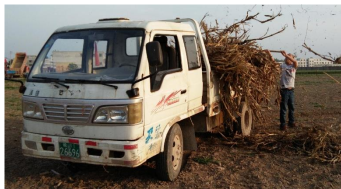
Fig.1 –The 5-ton farming truck used as the test vehicle
