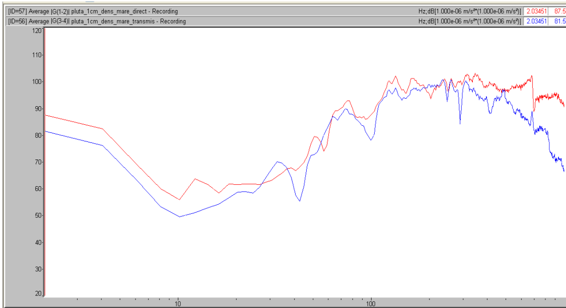
Fig.3 - Power flow vibration spectrum corresponding to the experiment from fig.2a, for sample of cork of 1 cm
