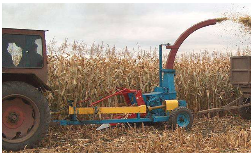
Fig. 5 - The aggregate tractor U650 with the combine CTF at harvesting of maize silage / Agregatul tractor U650 cu combina CTF la recoltat porumb siloz
