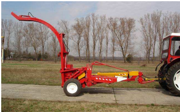
Fig. 2 The aggregate tractor U650 + trailed combine of forages CTF-65 / Agregatul tractor U650 + combina tractată de furaje CTF-65
