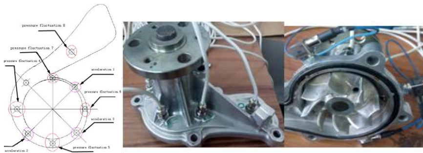
Fig.2- Layout of test points and image of sensor installation
