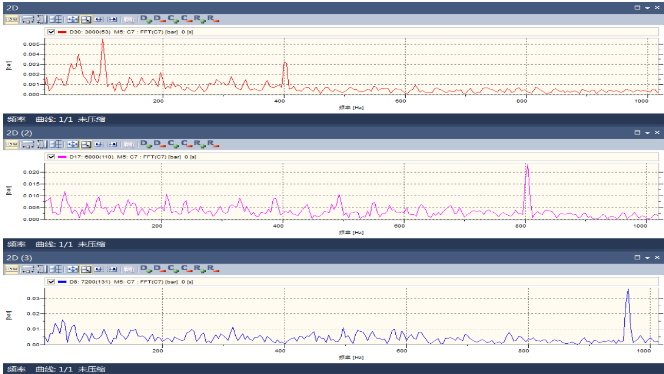
Fig.10-Pressure fluctuation at C7 under different working conditions
