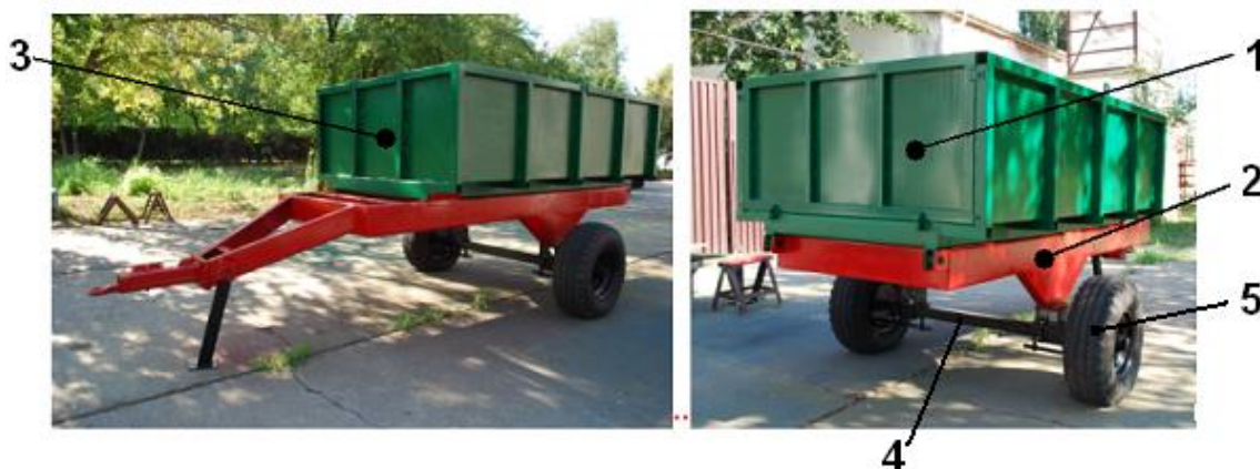
Fig. 1 – Stand for tyre testing, STP, equipped with tyres for testing 1. shutter; 2. assembled chassis; 3. body shell; 4. drivetrain; 5. tyre to be tested
