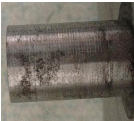
Fig.2- Universal joint journal with surface peeling and evident indentation
