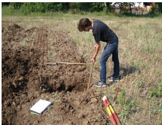
Fig. 2 – Determination of working depth by gauge tape
