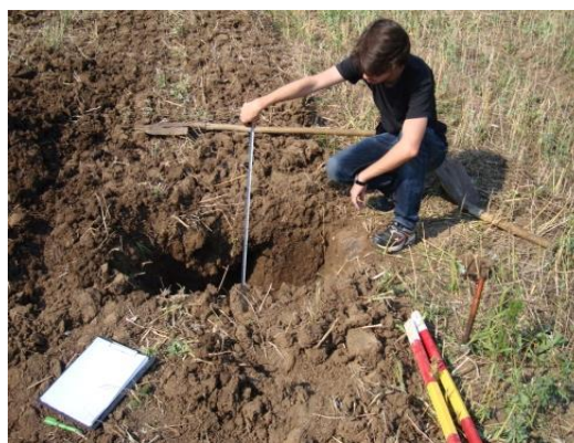
Fig. 2 – Determination of working depth by gauge tape
