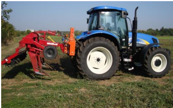
Fig. 1 – Equipment designed to soil deep loosening- EAA 220 in aggregate with a) New Holland T6070 tractor; b) Agrotron L 720 Deutz - Fahr tractor
