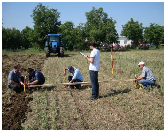
Fig. 4 – Determination of soil loosening degree
