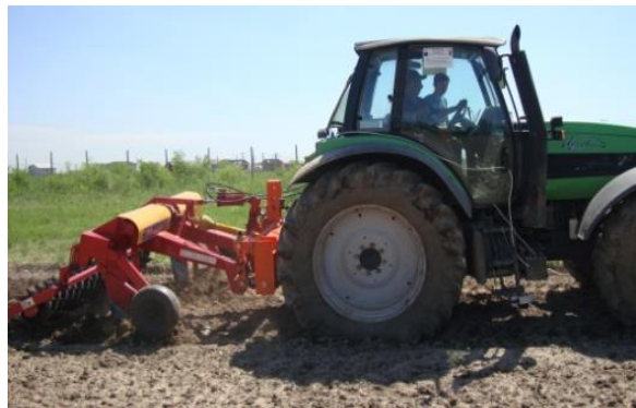
Fig. 1 – Equipment designed to soil deep loosening- EAA 220 in aggregate with a) New Holland T6070 tractor; b) Agrotron L 720 Deutz - Fahr tractor
