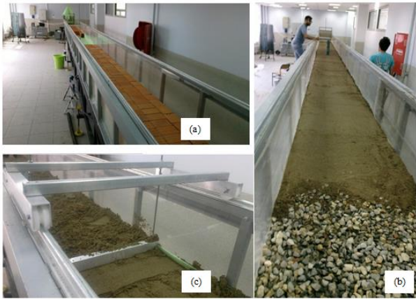
Figure 3: (a): Arrangement of the bricks along the flume, (b): The coarse gravels at the entrance of the flume, (c): The mobile system used to form the bed slope.
