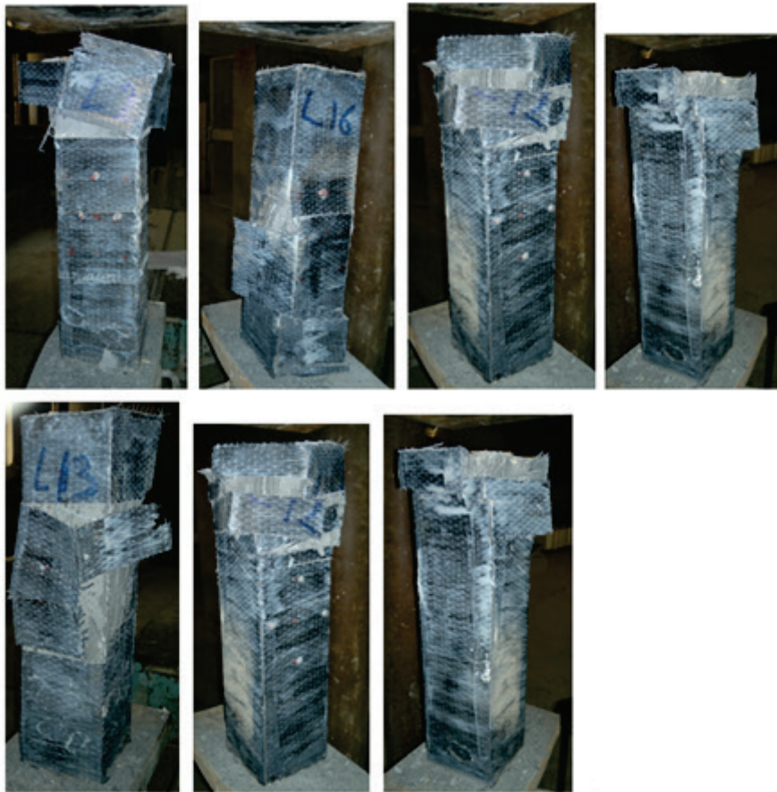
Photo (3): Failure of specimens of three groups.
