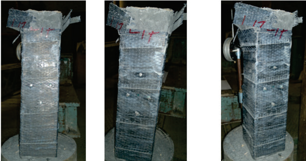
Photo 2: Details of distribution of demec strain devices
